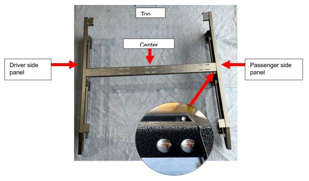
Step 1. Working on padded surface. Install the driver & passenger side panels onto the center cross bar, using the supplied M8 carriage bolt, M8 flat washers, M8 split washers, & M8 hex head nut. Do not tighten hardware until all cross bars are installed to prevent the bed rack from shifting. Repeat step for remaining crossbars.
