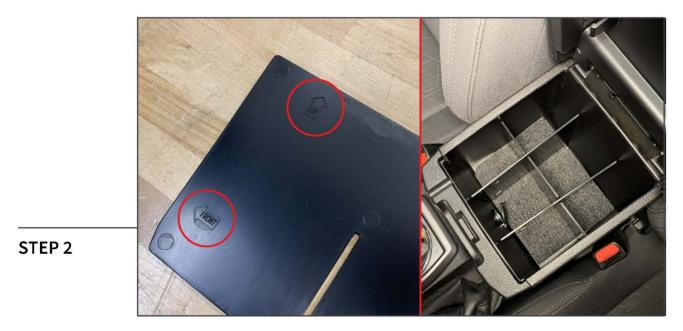
Place the (2) horizontal panels into the slots in the vertical panel, ensuring the panels are in the proper direction using the arrows. Press down until the horizontal panels are flush to the bottom of the center console.
