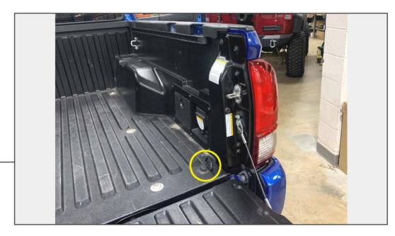
Remove (1) T-40 Torx bolt from the floor of the bed.
