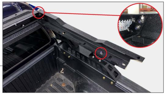
Install the rack side bar to the vehicle using (4) M8x1.25 x 20mm Allen bolt, (8) M8 flat washers, and (4) M8 lock nuts. Do not fully tighten hardware to allow adjustability.
