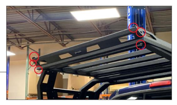
Install the rear rack panel to the vehicle using (6) M8x1.25 x 20mm Allen bolts, (12) M8 flat washers, and (6) M8 lock nuts.
