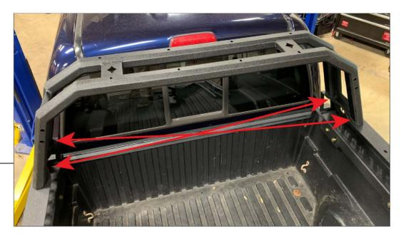
Install the (1) crossover roll bar to the side base panels using (4) M10x1.50 x 20mm Allen bolts, (8) M10 flat washers, and (4) M10 lock nuts. Do not fully tighten hardware to allow adjustability.
