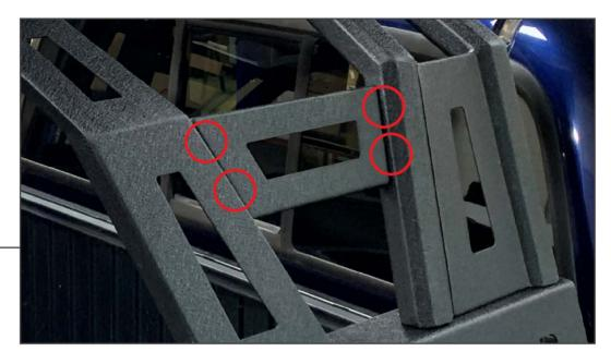
Install the connector panel to the crossover bar and the rear panel using (4) M8x1.25 x 20mm Allen bolts, (8) M8 flat washers, and (4) M8 lock nuts. Do not fully tighten hardware to allow adjustability.
