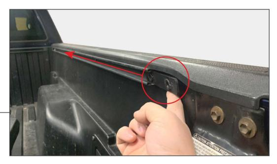
Remove the utility rail end cap. Slide (2) nut plates into the utility rail towards the front of the vehicle.
