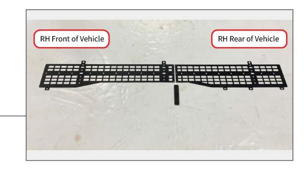
Assemble the molle panels using (1) nut plate, (6) M6 x 20mm Allen bolts, (6) M6 lock washers, and (6) M6 flat washers.
