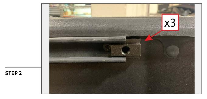
Remove the end cap from the bed utility rail. Insert (3) utility rail threaded inserts into the bed rail.
