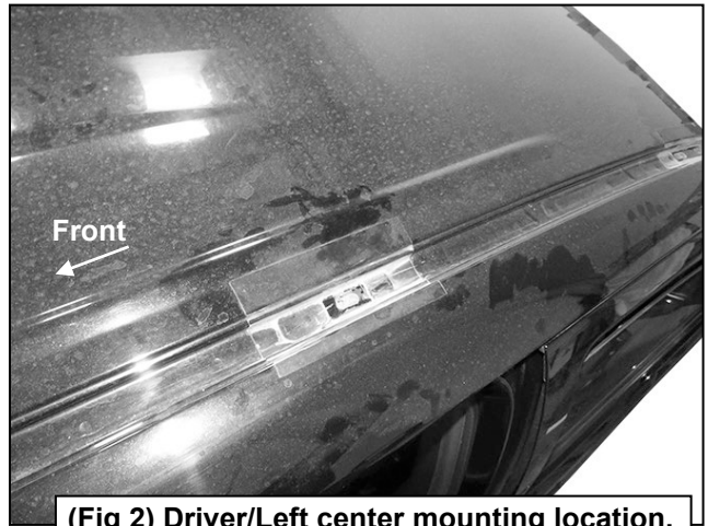
(Fig 2) Driver/Left center mounting location. Remove the factory rubber strip in the rain gutter to access the mounting locations
