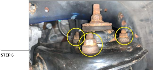
Remove (3) 14mm nuts from the upper strut assembly.
