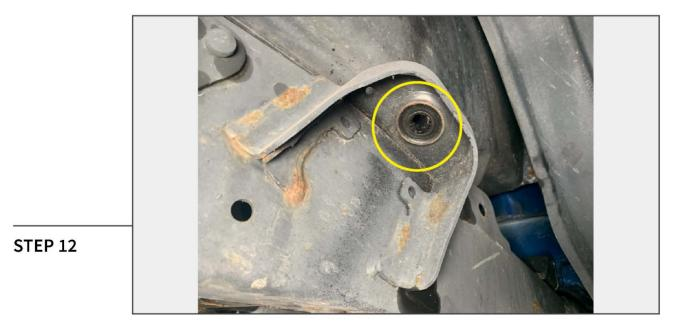
Inspect the upper shock absorber mount to ensure no hardware is stuck to either side of the frame. Remove any stuck hardware if applicable.
