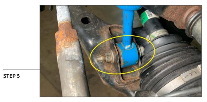
Remove (1) 21mm bolt from the bottom of the strut assembly.
