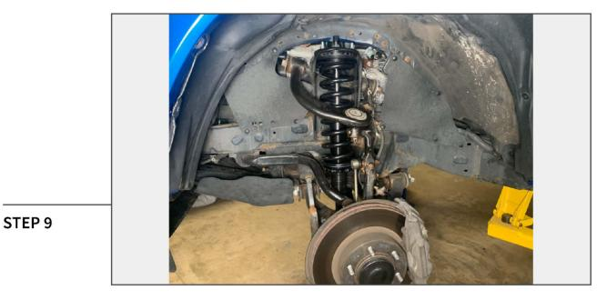
Re-assemble the vehicle suspension following steps 1-8 in reverse order using original hardware.
