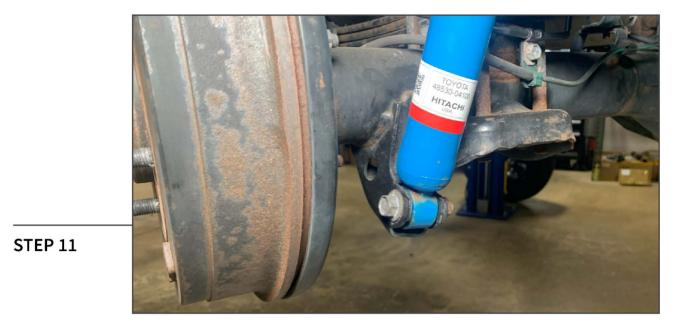
Remove (1) 17mm bolt from the bottom of the shock absorber. Remove the shock absorber from the vehicle.
