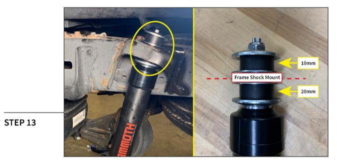
Install the top of the shock absorber to the frame mount using the provided hardware and bushings.
