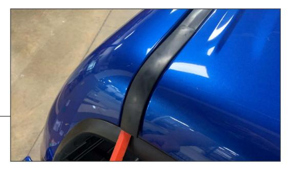
Using a plastic panel removal tool, remove the weatherstripping from both sides of the roof. Pry starting from above the rear window to remove the corner weatherstrip. Pry up on the remaining weatherstrip to remove the weatherstripping from the roof of the vehicle.
