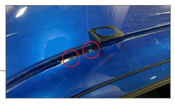
Using the front bolt holes, secure the roof bracket to the vehicle using (2)  $M6x1.00 \times 25mm$  Allen bolts and (2) M6 rubber flat washers.
