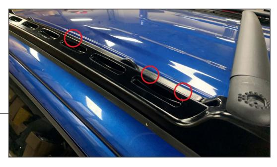
Clean the weatherstrip track above the rear window using the provided (2) alcohol wipes. Peel back and adhere the double sided tape weatherstrip attached to the roof rack to the vehicle. Secure the rear of the roof rack using (3) M6x1.00 x 45mm bolts and (3) M6 rubber flat washers. Tighten all roof rack hardware.
