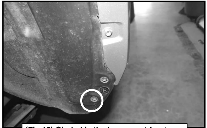
(Fig 16) Circled is the lowermost front bolt which will need to be saved for later
