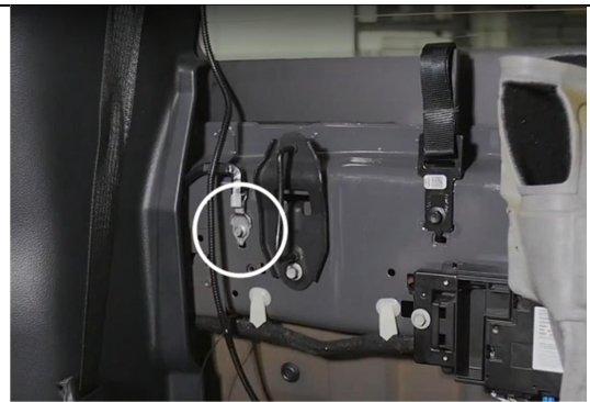
Attach black ground wire to the 8mm stud circled above. 5
