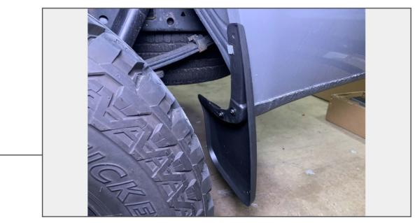
Secure the mud guard using (2) Phillips screws and (2) flat washers. Secure the upper portion of the mud guard using (1) spring clip, ensuring the clip attaches to the mud guard and the vehicle fender
