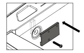
2. Screw the outer block to the large aluminum square pc, screw well and do not tighten.
