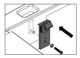
2. Close the cover, move the adapter tongue to match the cover latch system. Adjust the cover position, to make sure the adapter tongue is in the Middle of cover aluminum groove.
