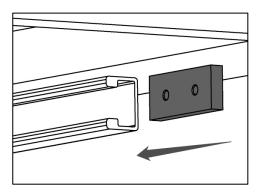
\*Attach the clamp bracket to the plate with the included Allen head bolts.
