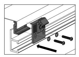
2. Close the cover, move the block, make sure the adapter tongue is under the cover latch system. Adjust the adapter, to make sure the tongue is in the Middle of cover aluminum groove
