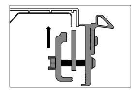
2. Close the cover, move the block, make sure the adapter tongue is under the cover latch system. Adjust the Adapter position to make sure the adapter tongue is in the Middle of cover aluminum groove.
