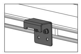
\* Secure Tri-fold Cover latches (Front Clamp Knobs) to these brackets.
