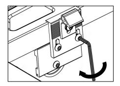
3. Close the cover, move the adapter tongue to match the cover latch system. Adjust the cover position, to make sure the Adapter tongue is in the Middle of cover aluminum groove. Make sure the lip of outer block is sit firmly on the bed rail, and tighten all screws/bolts.
