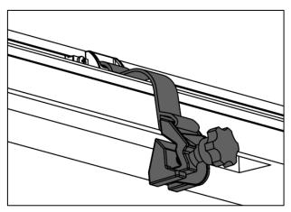
When the front clamps are secured, install the safety strap (see the photos). Tighten the knob of the safety straps.
