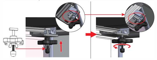
Take out the safety hook and hook it on the side rail fixing block.
