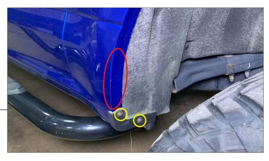
Clean the designated area on the fender with exterior detailer/isopropyl alcohol. Remove the (2) 5.5mm bolts on the fender.
