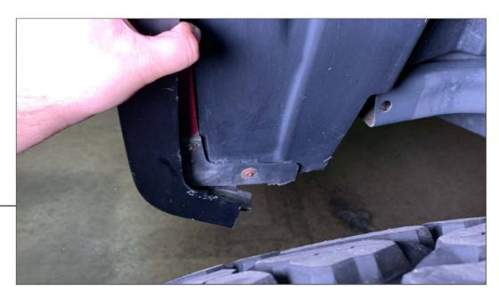
Remove the (1) push clip at the bottom of the fender flare, pull it away enough to remove the (1) Phillips screw in the fender liner.
