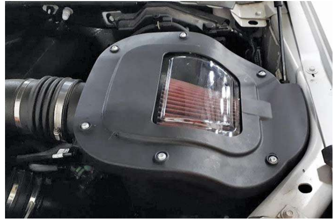
13. Clip the harness and vacuum line into position on the air box bracket.
