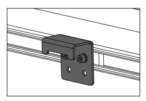
\*Line the bracket up with the tri-fold cover clamp location once they are lined up. Secure bracket to the vehicle bed rail.
