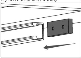
\*Attach the clamp bracket to the plate with the included (2) Allen head bolts.
