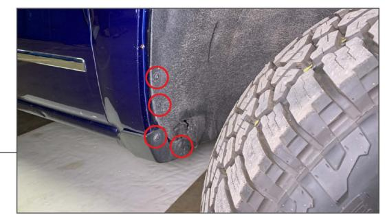
Remove (4) T-15 Torx screws from the fender liner.
