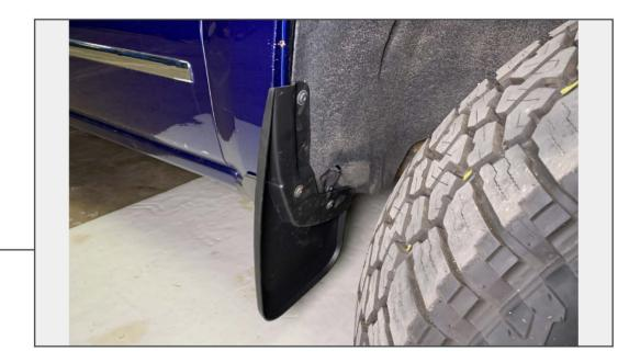
Align the mud guard to the vehicle fender, and secure into place using the original (4) T-15 Torx screws.
