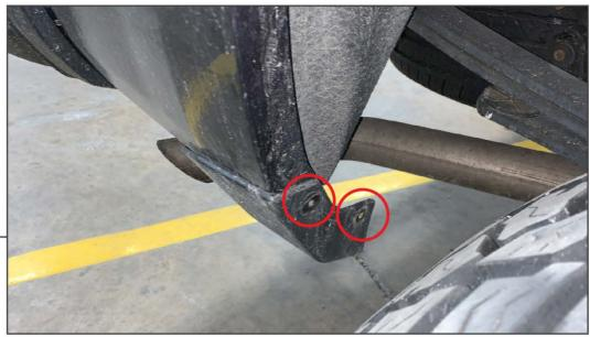
Remove (2) T-15 Torx screws from the vehicle.
