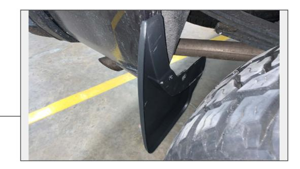
Align the rear mud flap to the vehicle. Secure the mud flap reusing the original (2) T-15 Torx screws.
