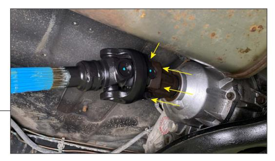
Fit the new driveshaft to the transfer case yoke, and secure using the (4) 6mm Allen bolts. Tighten all bolts evenly until secure.
