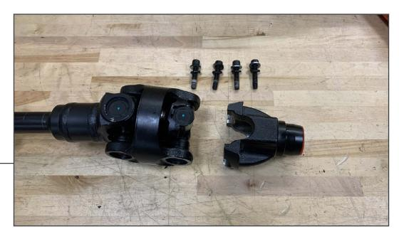
Remove the (4) 6mm Allen bolts from the new driveshaft yoke. Remove the pre-installed plastic cap.
