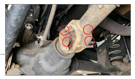
Remove the (4) 5/16" bolts and U-Joint caps from the front differential yoke to disconnect the driveshaft from the differential.
