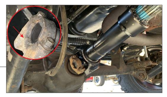
Extend/retract the driveshaft as necessary to fit the U-Joint end caps into the rear pinion. Ensure each end cap is properly fitted into the pinion, and are not over-lapping the stopper on each side. Secure the front of the driveshaft using the original (4) 5/16" bolts and end caps. Tighten all bolts evenly until secure.
