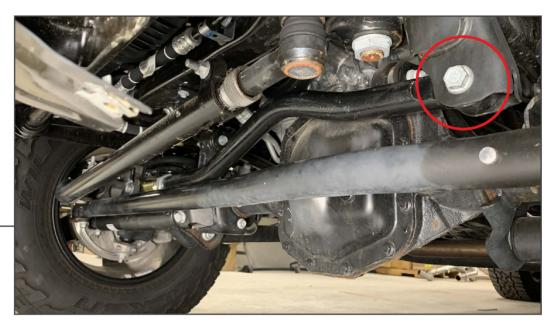
Fit the track bar to the vehicle frame using the original (1) 21mm bolt and nut. Do not fully tighten the hardware.
