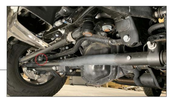
Remove (1) 21mm bolt and flag nut from the vehicle axle mount. Remove the original track bar from the vehicle.
