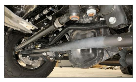
Tighten the jam nut to secure the adjustment. Torque all of the track bar bolts to 125 ft. lbs.
