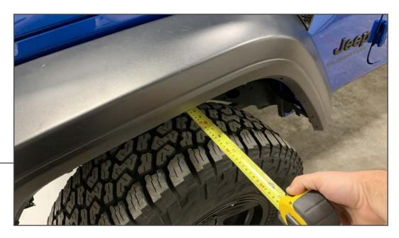
Park the vehicle with the steering wheel straight. Measure the distance from the upper shock aborber mount to the outer edge of the fender flare on each side of the vehicle to determine the center-point of the vehicle.
