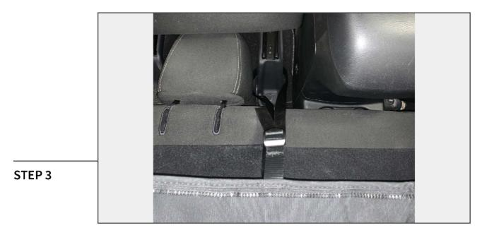
Route the (2) inner straps towards the inner front seat bracket. Wrap each strap around the seat bracket, and loosely secure the tonneau extension into place.
