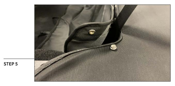
Tighten all mounting straps evenly until secure. With the straps secure, use a Phillips screwdriver to fit the (5) button screws into the tonneau cover in order to utilize the button snaps in the tonneau cover extension. Install the (5) screw caps over the button screw threads.
