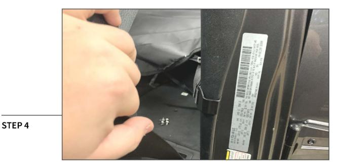
Route the (2) outer straps with hooks towards the front door jam. Attach the hook to the front door jam.
