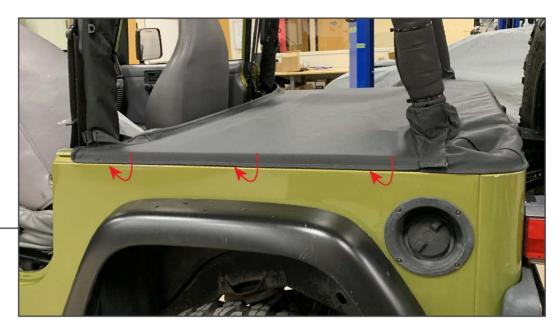
Tuck the plastic along the inner edge of the tonneau cover under the vehicle side lip on both sides of the vehicle.
