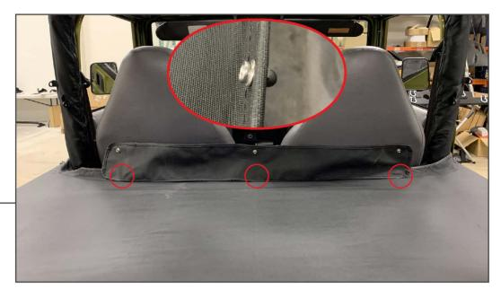
Merge Panel: If installing a windbreaker (SKU: J174543), add the merge panel to the front of the tonneau cover using (3) button head screws, (6) rubber grommets, and (3) plastic nuts. Ensure to use the windbreaker as a template to ensure proper placement. Insert the screws through the tonneau cover material using a Phillips head screwdriver.
