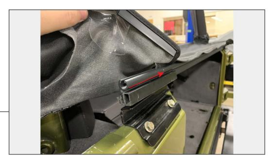
Under the rear of the tonneau cover, locate the rod flap. Feed the rod flap through the tailgate bar.
