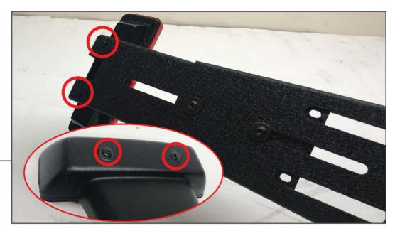
Remove the (2) 3rd brake light screws from the original tire mount using a Phillips screwdriver. Once removed, reinstall the light and screws into the new mount.
