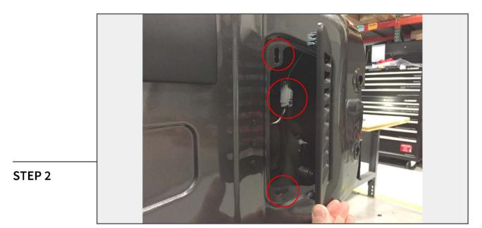
Open the tailgate to access the 3rd brake light connector. Remove the interior vent cover with a panel removal tool. Unclip the brake light wiring harness. Close the tailgate, do not install the interior vent cover.
