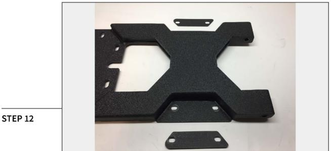
Place the thin spacer behind the upper tire carrier bracket mount, and the thick bracket behind the lower tire carrier bracket mount.
