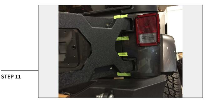
Install the tire carrier bracket to the hinges using the supplied hinge pins. Once installed secure the hinge pins using the provided c-clips. \*\*Note: A rubber mallet may be needed to seat the hinge pins.
