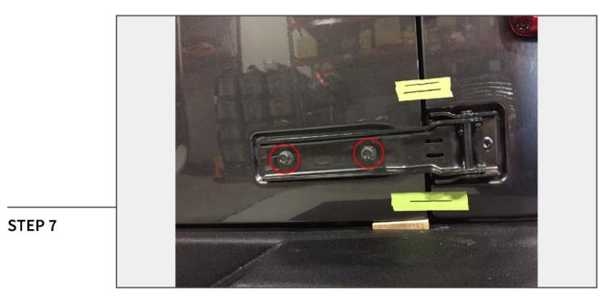
Remove the plastic hinge covers followed by (2) 13mm bolts securing the hinge each hinge to the tailgate.
