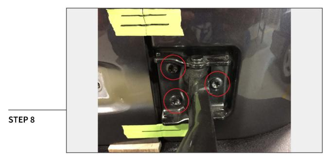
With the hinges unbolted from the tailgate, open the hinge to access the (3) T-50 Torx bit bolts.
