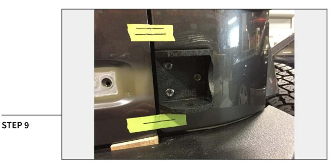
Attach the supplied hinge mounts using the factory T-50 Torx bolts. Tighten the bolts down in several passes, they will self-center.
