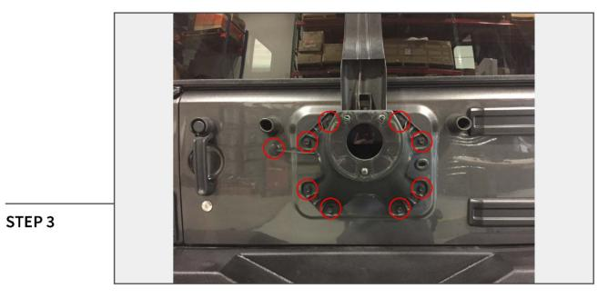
Remove the (8) 13mm bolts holding the factory tire carrier in place. Remove the 3rd brake light wiring grommet to remove the plug from the vehicle.
