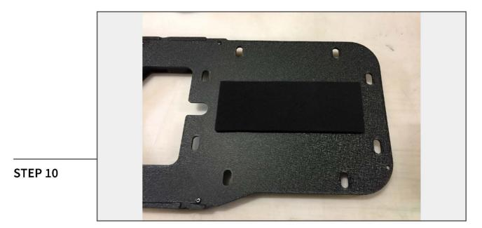
Install the foam cover for the air vent hole. Remove the double sided tape backing on all (4) corners. Install the foam to the tire carrier bracket.
