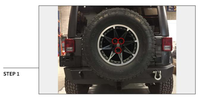
Begin by removing the spare tire by removing the (3) lug nuts.
