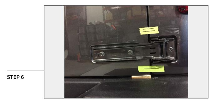
Shim the bottom of the tailgate to prevent it from sagging when the hinge bolts are removed.
