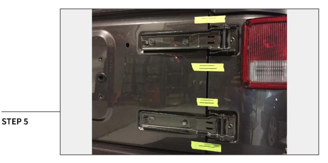
Apply painters tape to the vehicle so that you can line up the tailgate correctly if need. Mark the tailgate in several locations. Use a straight edge to mark the tape as a visual reference. Use a razor blade to cut the tape in half at the seam.
