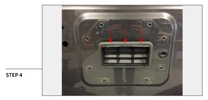
Using a panel removal tool, remove the factory air vent.
