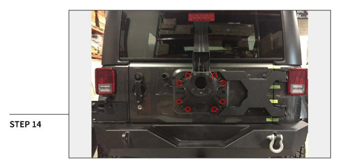
Install the factory tire carrier on top of the tire carrier bracket using the factory hardware.
