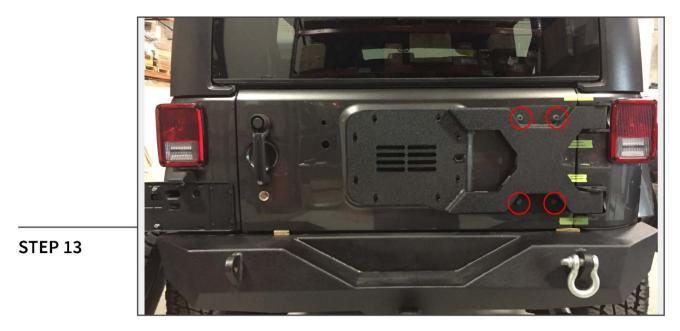
Use the factory hinge bolts to secure the tire carrier bracket to the tailgate. Ensure the reference marks made earlier still line up prior to tightening the tire carrier bracket.
