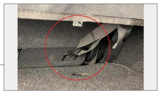
Clip the bottom hook straps into the anchor point on the base of the rear seat.
