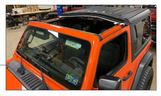
Unlock the factory freedom panels and remove the panels from the vehicle.
