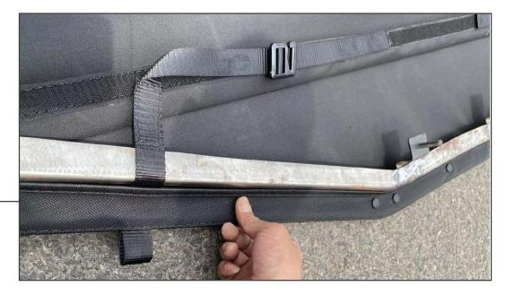
Begin by unrolling the cover. Place the metal frame on top of the cover. Starting at the rear of the cover, tuck the frame into the cover pocket and button the cover to the frame. Secure into place using the pre-installed snaps.
