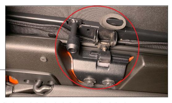
Open the sunroof latches. Fit the hook under the freedom panel header brackets.
