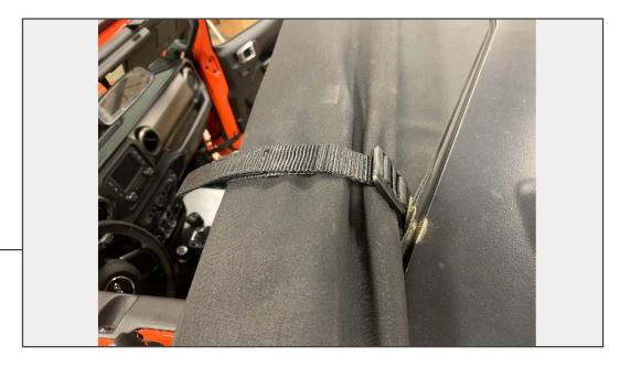
To open the sunroof, unlatch the latches and roll the sunroof backwards. Use the Velcro straps to secure the sunroof in the open position, place the plastic clip through the top loophole and pull the strap tight.
