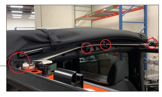
Place the sunroof assembly onto the vehicle hardtop. Ensure to overlap the sunroof over the hardtop freedom panel gasket to ensure proper fitment. Fit the pre-installed M8 bolts through the freedom panel mount holes.
