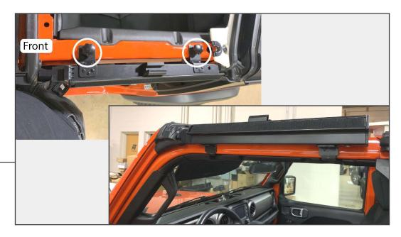
Install the sunroof brackets to the vehicle roll bars. Use the long thumb screws removed in step 2, align the brackets with the holes in the factory roll bar. Carefully align the thumb screw and secure the brackets to the vehicle. Repeat this on both sides.
