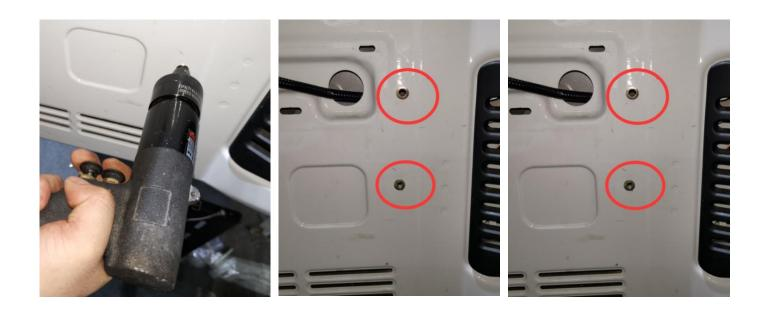
**Step 4:** Install the tailgate table with supplied bolts.
