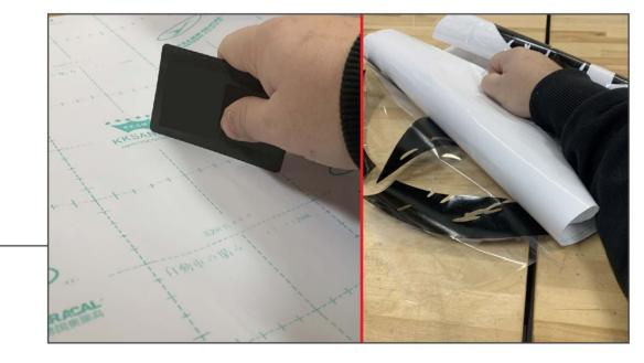
Using a plastic card, press the vinyl decal onto the transfer tape. Once pressed down, peel the release paper to reveal the decal on the transfer tape.
