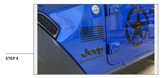
Place the decal onto the vehicle and adjust as necessary. Once adjusted, squeegee the decal into the vehicle panel to remove the remaining soapy water solution and promote proper adhesion. Peel the transfer tape from the decal, ensure the decal is properly adhered.
