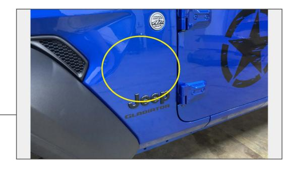
Clean the vehicle of dust/dirt in the area where the decal is desired using isopropyl alcohol and a microfiber cloth.
