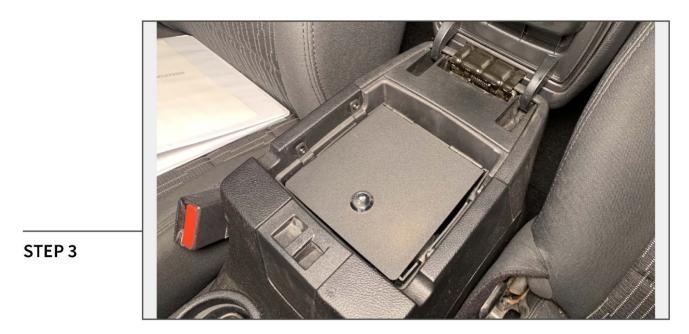
Close the lock vault lid, and secure into place using the provided keys.
