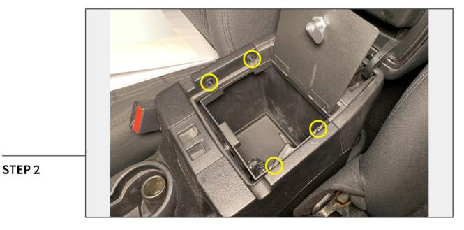
Place the lock vault into the center console with the lid open. Secure the lock vault using the (4) provided Phillips head screws. Tighten the hardware evenly until secure.
