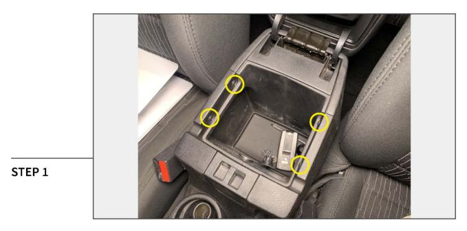
Remove (4) T-20 Torx screws from the center console.
