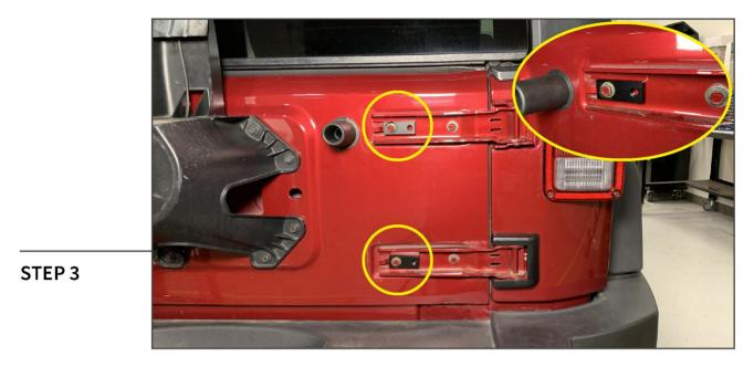
Place the (2) threaded blocks within the tailgate hinge and secure using the original (2) 13mm bolts.
