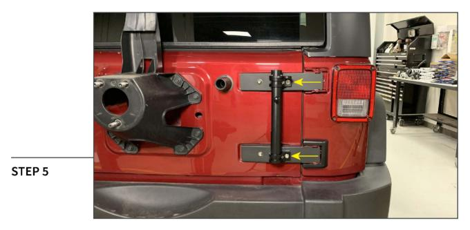
Install the flag pole mounts and the flag pole to the vehicle together, and tighten the mounts to the tailgate hinge brackets using (2) M10 x 12mm Allen bolts.
