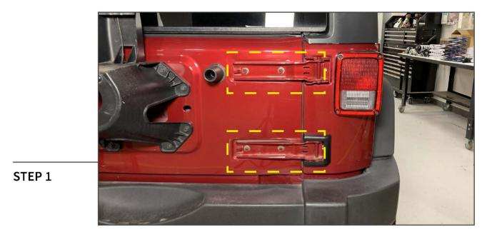
Remove the inner hinge covers from the tailgate using a plastic panel removal tool.
