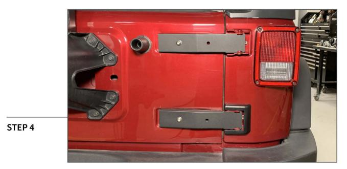
Install the included (2) tailgate hinge brackets to the tailgate hinges using (2) M10 x 20mm Allen bolts and (2) M10 flat washers. Tighten until secure.
