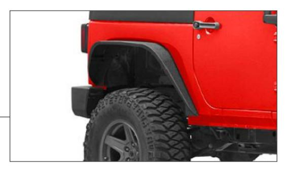
Ensure all M6 hardware is tightened to 8 ft-lbs and all M8 hardware is tightened to 18 ft-lbs. Repeat steps 1-7 to the opposite side of the vehicle.
