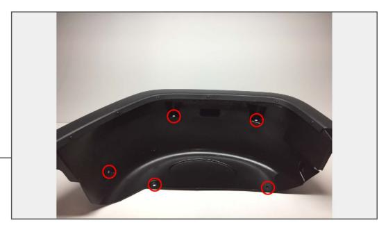
Using a flat head screw driver or trim panel removal tool, remove the (5) push clips holding the rear fender liner to the vehicle. Then, firmly pull the stock fender away from the vehicle moving from front to back. Some of the factory plastic clips may break when removing the fenders, this is normal.
