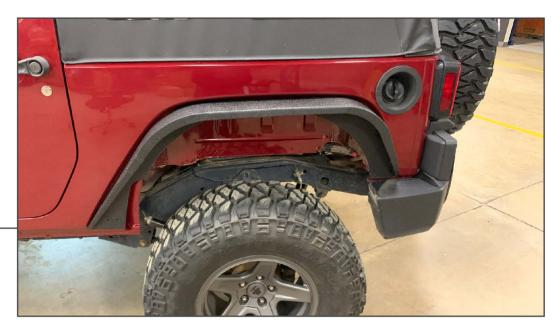
Install the fender using (6) M6 Allen Bolts, (6) M6 Flat Washers, (6) M6 Lock Washers.
