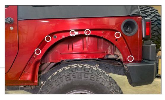
Enlarging the (6) factory holes circled above using a 25/64" drill bit. Paint any exposed metal with touch up paint or clear nail polish. Then install the provided rivnuts into the enlarged holes. Reference Step 2 as needed.
