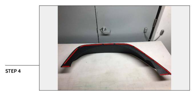
Install the supplied foam to the fender before installation.
