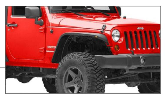
Ensure all M6 hardware is tightened to 8 ft-lbs and all M8 hardware is tightened to 18 ft-lbs. Installation is now complete. Repeat steps 1-11 to the opposite side of the vehicle.
