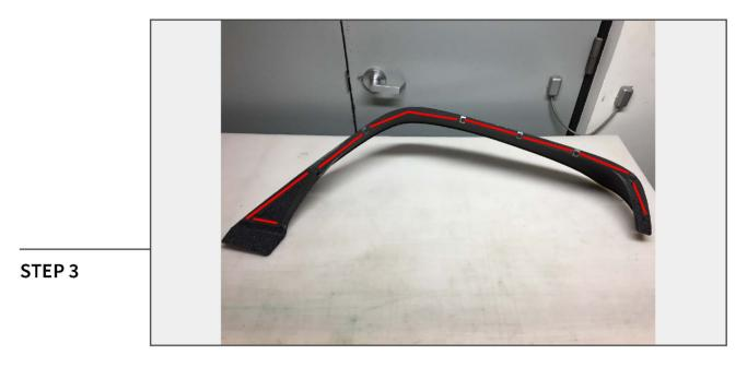
Install the supplied foam on the back side of the fenders, as shown above.
