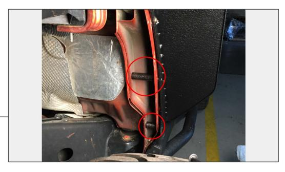
Install the supplied spacers between the inner and outer fenders using the M8 x 1.25 120mm bolt for the long spacer and the M8 x 1.25 65mm bolt for the shorter spacer. Secure the bolts with lock washers, flat washers, and nut.
