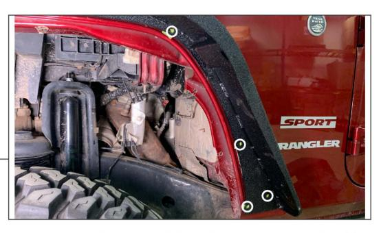
Loosely install the fender flare using the provided M6 Allen bolts. Using a marker, mark the (4) additional holes that will need to be drilled. Then remove the fender.
