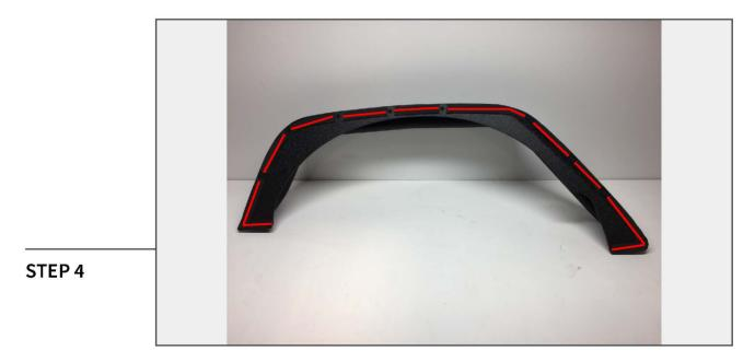
Install the supplied foam to the fender before installation.
