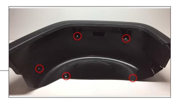
Using a flat head screw driver or trim panel removal tool, remove the (5) push clips holding the rear fender liner to the vehicle. Then, firmly pull the stock fender away from the vehicle moving from front to back.
