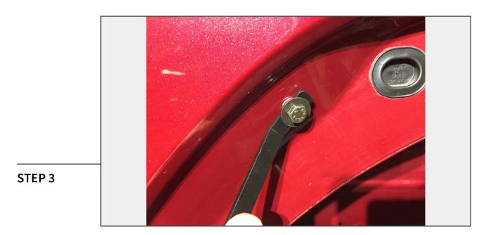
Using the supplied handle and long M6 x 1.0, install the rivnuts. Hold the rivnut in place with the handle and tighten the rivnut securing it to the vehicle.
