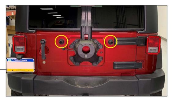
Remove the (2) rubber spare tire bumpers from the tailgate by firmly pulling away while twisting outward.
