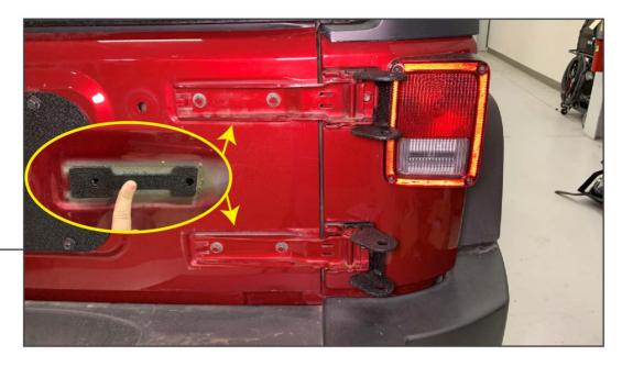
Place (1) provided hinge bracket under each vehicle hinge assembly. Secure the brackets and hinges using original hinge assembly hardware. Install (1) hinge spacer under each bracket attaching the hinge to the tailgate, then tighten using original hardware. Re-install hinge covers if desired.
