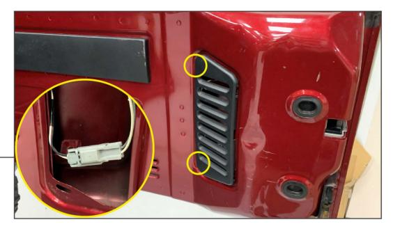
Gently pry along the (2) metal clips to remove the plastic trim cover from the tailgate. Un-plug the third brake light connector from the vehicle.
