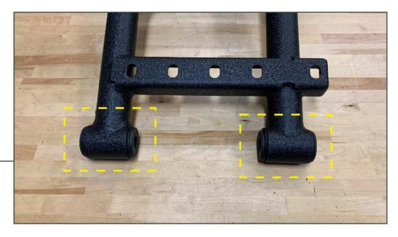
Install (4) tire carrier bushings into the tire carrier.
