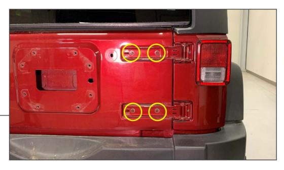
Ensure the tailgate is closed. Remove (4) 13mm bolts from the tailgate hinges.
