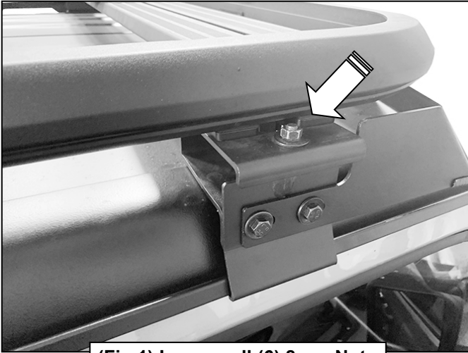
(Fig 1) Loosen all (6) 8mm Nuts on top of the clamp brackets
