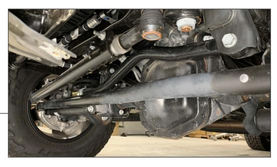
Tighten the adjustment clamps to secure the adjustment into place. With the vehicle on the ground, torque all of the track bar bolts to 125 ft. lbs.
