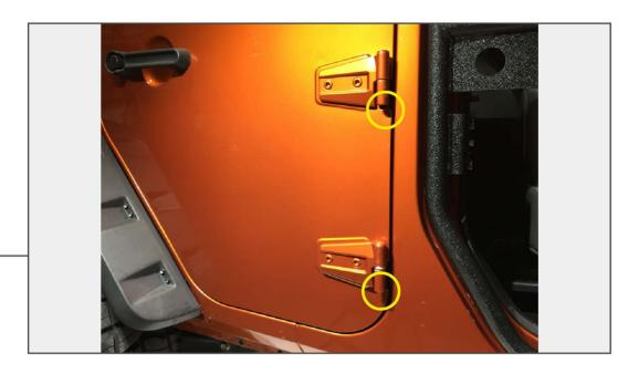
Remove the T-50 Torx nut from the bottom of each door hinge.
