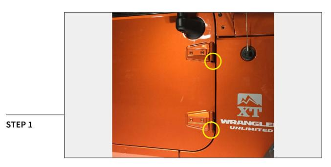
Remove the T-50 Torx nut from the bottom of each door hinge.
