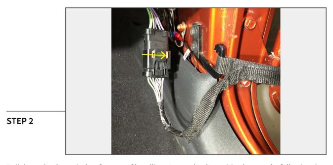
Roll down the door window for ease of handling. Access the door wiring harness by following the lead from the door towards the dashboard. Slide the red locking tab, then depress the black tab to disconnect the electrical connection. Lift the hinge strap from the chassis mount. With a firm grip, lift and remove the door from the vehicle.
