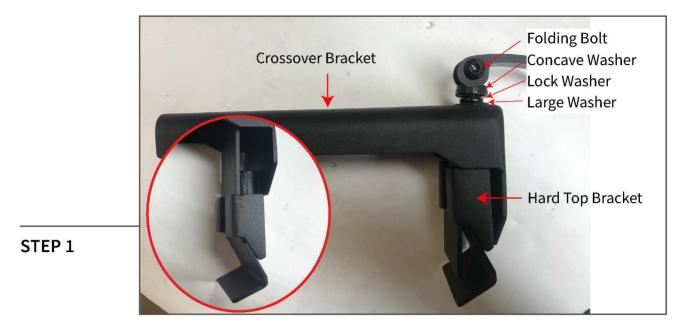
Begin by assembling the roof brackets by using (1) crossover bracket and (1) hard top bracket. Slide the hard top bracket onto the crossover bracket, then install (1) M10x1.50 Folding bolt, (1) concave washer, (1) M10 lock washer, and (1) M10 large (25mm diameter) flat washer to secure the two brackets together. Do this for all provided brackets.
