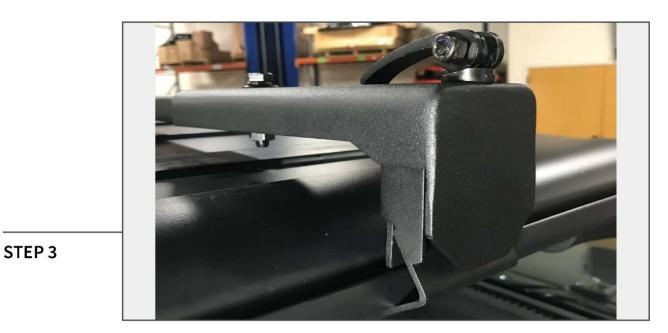
Install brackets onto hard top by sliding the lower portion into the channel. Tighten the folding bolt snug, but do not flip the handle over. Do this for all four brackets.
