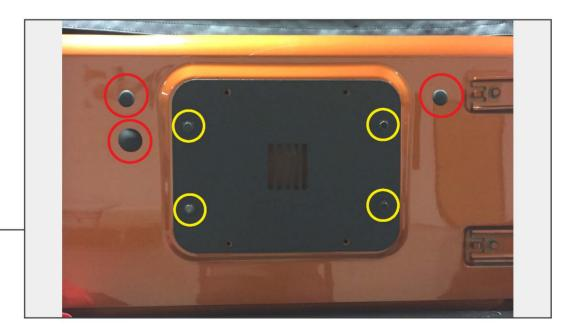
Loosely install the rear plate to the tailgate re-using the original (4) 13mm bolts. Install the (2) small grommets into the previous spare tire bumper holes in the tailgate. Install (1) large grommet into the third brake light wiring harness hole in the tailgate.
