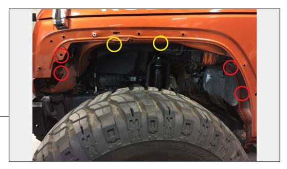
Remove (2) 10mm bolts and (4) plastic push clips from the original inner fender liner.
