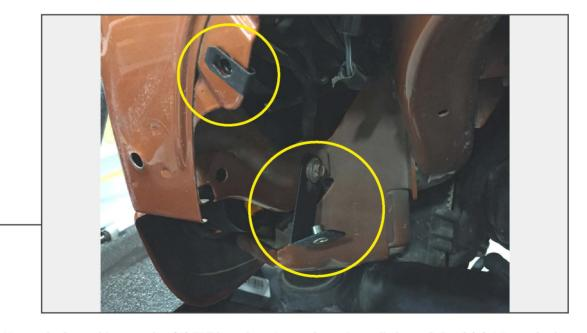
Remove (1) 10mm bolt and insert the (1) "L" bracket. Loosely re-install the original (1) 10mm bolt. Slide (1) clip nut onto the vehicle at the designated location.
