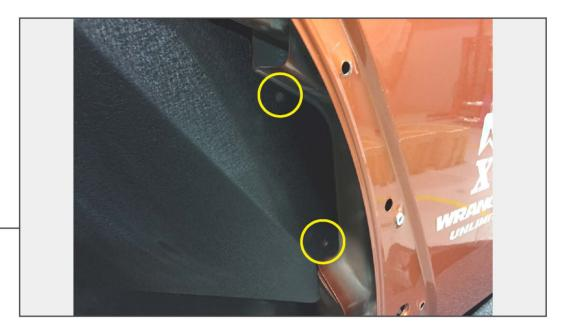
Loosely install the inner fender liner using (6) Allen bolts. Using a permanent marker, mark the hole locations on the rear most holes. Once indicated, remove the fender liner. Tighten the front "L" bracket.
