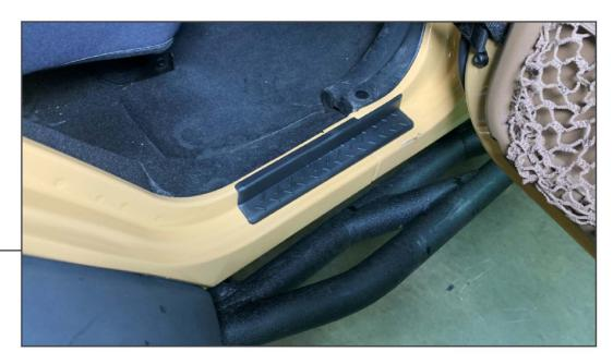
Peel back the double sided tape backing from the entry guard. Firmly adhere the entry guard to the vehicle. Repeat steps 1-2 to all remaining door entry areas of the vehicle.
