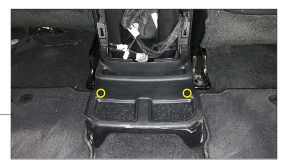
Lift the center console assembly as much as possible. Reach under the storage tray and remove (2) T-20 Torx screws. Reference the new cup holder to approximate the screw locations.
