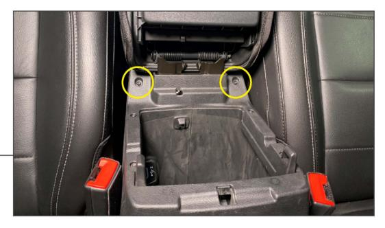
Engage the vehicle emergency brake. Lift the center console lid. Remove (2) T-20 Torx screws behind the backside of the lid.
