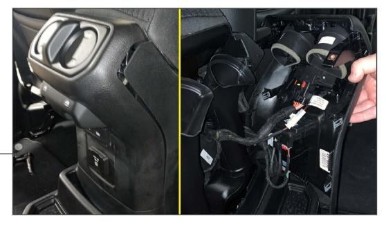
Using a plastic pry tool, pry the upper portion of the center console away from the center console assembly. Unplug the various electrical connectors. Set panel aside.
