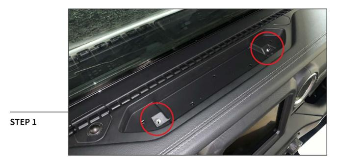
Remove the rubber mat from the dashboard. Remove (2) Phillips screws from the dashboard.
