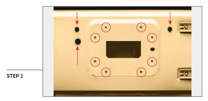
Unplug the tire carrier wiring harness from inside the tailgate, and pull the wiring harness through to the outside of the tailgate. Then, remove the spare tire carrier by removing (8) 13mm bolts, if necessary.
