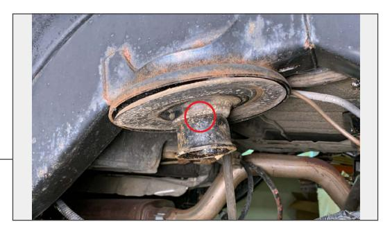
Remove the foam bump stop from the bump stop cup, then remove (1) 16mm bolt to remove the bump stop cup from the frame.
