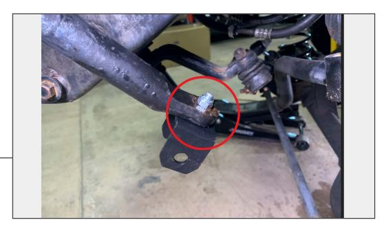
Install the sway bar link adapters to the bottom of the sway bar using provided  $5/16 \times 1.25$ " bolts, lock nuts, and washers.
