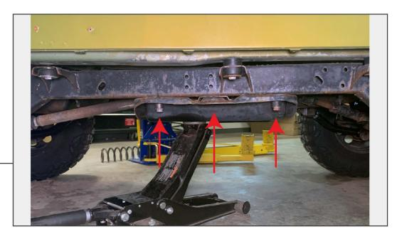
Loosen but do not remove the (6) transmission skid plate bolts from the frame of the vehicle using a 19mm socket.
