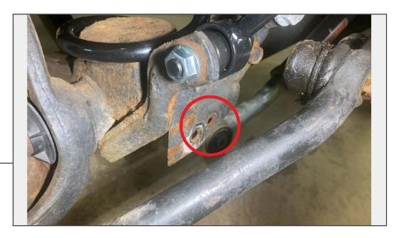
Drill one hole in the axle track bar mount. Measure 1" from the center of the original track bar mounting hole. Secure the track bar to the axle using provided (1) M10x65mm bolt, lock washer, flat washer, and nut. While the tires are on the ground, turn the steering wheel to move the body with the track bar. Once aligned, insert the bolt.
