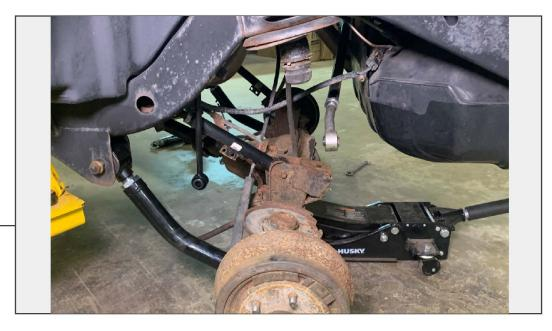
Slowly lower the axle down with the floor jack to remove the coil springs.
