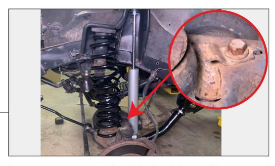
Install the new coil spring and spring spacer into the vehicle. Align the bottom of the spring into the cutout in the axle housing, then reinstall the spring clip to secure the spring into place.
