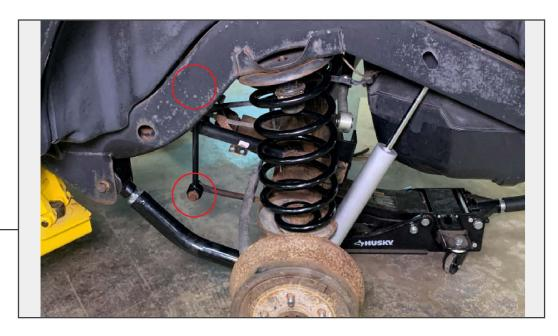
While the vehicle is on the ground, install the provided rear sway bar links onto the vehicle reusing original hardware.
