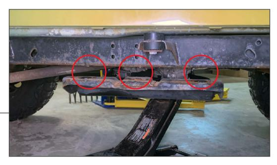
Insert the (3) transfer case drop pucks per side in between the skid plate and the frame of the vehicle. Loosely install (3) provided tapered bolts into the frame. Then repeat procedure to opposite side. Tighten all skid plate bolts once both drop brackets are into place.
