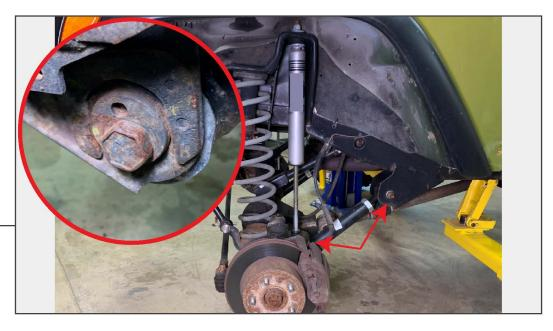
Mark the cam on the lower control arm bolt with the axle housing, then loosen the (2) 21mm control arm bolts.
