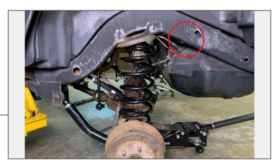
With the axle lowered, install the coil springs onto the axle mount. While ensuring the springs are aligned within the axle and the frame, lift the rear axle up with the floor jack to hold the springs in place. Install the shock absorber into the frame reusing original hardware.
