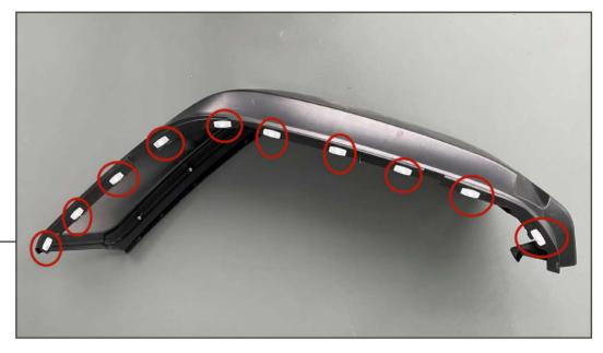
Install the provide fender clips.
