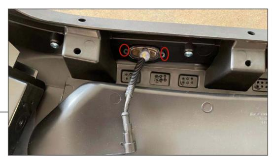
Install the smoked side marker lights using the provided self tapping screws.
