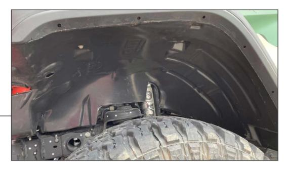
Connect new lights to the original wiring connector. Install provided fender liner using included clips and original hardware.
