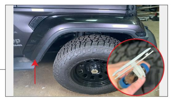
Using pliers, depress the white fender clips while pulling the fender away from the vehicle. Start at the bottom of the fender closest to the doors and work your way forward.
