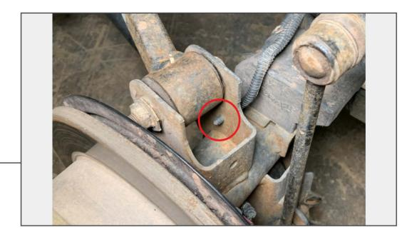
Remove the wiring harness from the control arm mount using a panel removal tool.
