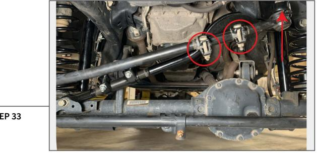
Loosen the (2) 15mm nuts on the drag link. Turn the steering wheel to point straight. Turn the adjustment sleeve until the ball-joint end of the drag link reaches the pitman arm. Reinstall the drag link to the pitman arm using original 21mm nut, and torque to 77ft-lbs.
