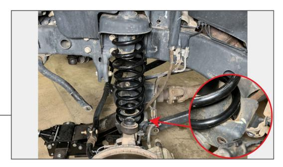
Install the new front spring (taller spring) onto the vehicle. Be sure to align the bottom of the spring with the cutout in the axle. Tighten the bump stop to the axle.
