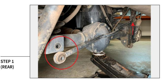
Using a jack and jack-stands, support the vehicle off the ground. Place the jack-stands under the frame rails of the vehicle. Remove the rear wheels. Support the rear axle using the floor jack. Remove the 21mm Track Bar bolt going through the axle. Loosen, but do not remove the 21mm Track Bar bolt through the vehicle's frame.
