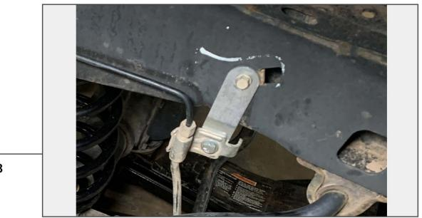
Gently massage the brake line to reach the bracket extension. Install the brake line extension to the brake line bracket. Bolt the extension to the frame using original hardware. Be sure the brake line is not touching anything.
