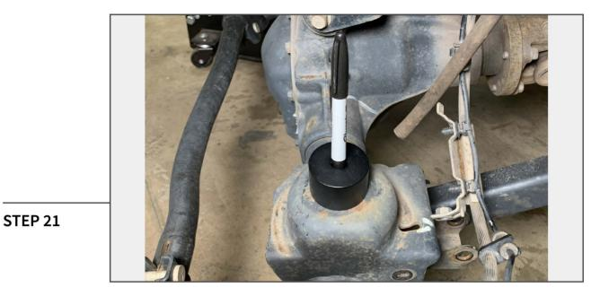
Using a permanent marker and the provided bump stop, make a mark onto the center of the spring perch for drilling. Drill this hole using a 3/8" drill bit.
