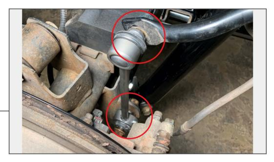
Install new sway bar links into the vehicle, use the provided lock nut to secure the sway bar link to the sway bar, then use the original hardware for fastening to the axle.
