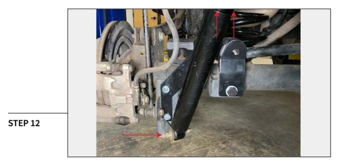
Install the rear shocks into the vehicle. Reuse the original hardware.
