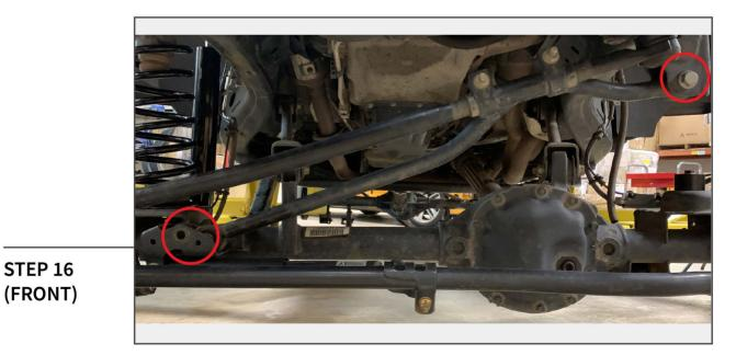
Using a jack and jack-stands, support the vehicle off the ground. Place the jack-stands under the frame rails of the vehicle. Remove the front wheels. Support the front axle with the floor jack. Remove the (2) 21mm track bar bolts from the vehicle. Remove the track bar from the vehicle.
