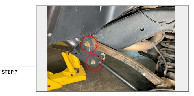
Loosen, but do not remove, the (2) 21mm control arm bolts from the frame.
