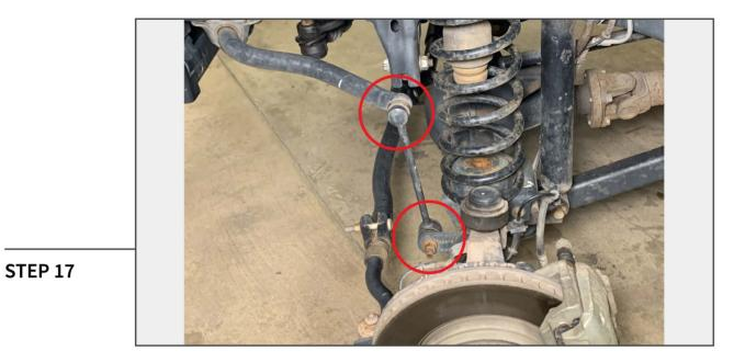
Remove the sway bar links from the vehicle. Remove the top 19mm nut, then the 18mm bolt from the bottom of the sway bar links.
