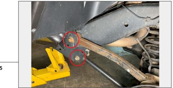
Reinstall wheels onto the vehicle. While the suspension is loaded, tighten the control arm bolts attached to the frame to 125 ft-lbs.
