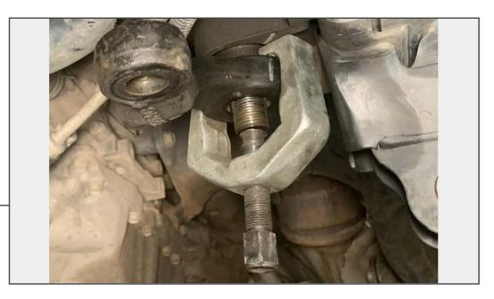
Using a pitman arm puller, align the puller claws around the pitman arm. Tighten the puller by hand until the screw aligns with the stud on the steering box. Tighten the puller until the pitman arm is removed from the steering box.
