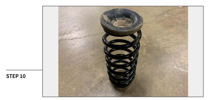
Remove the spring isolator from the old spring, and place it on top of the new spring in the same orientation. Install the rear spring (shorter spring) into the vehicle.
