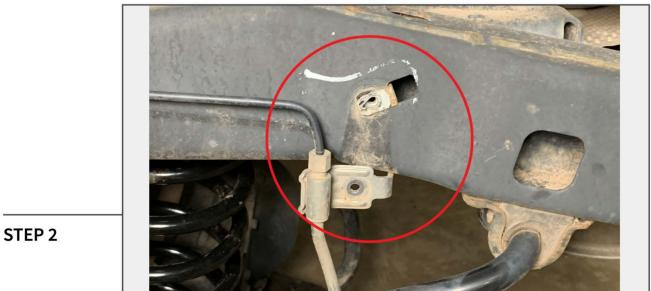
Remove (1) 10mm bolt to remove the brake line from the frame. This will allow additional clearance when lowering the axle. Repeat on both sides of the vehicle.
